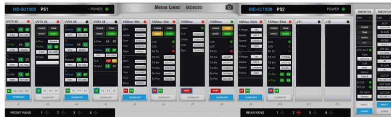
NetGazer® provides visual views of networks, services, equipment racks, chassis and line cards. Start at a high level of visualization and then drill down to specific signal parameters to isolate and resolve issues fast.
