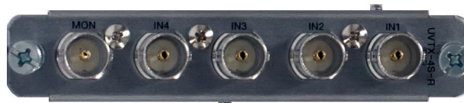
MD8000 – UVTX-2022 (SDI) – Electrical Rear Board Connectors
