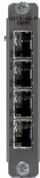
UVTX/UVRX H264 SFP Rear Panel (Optical)
